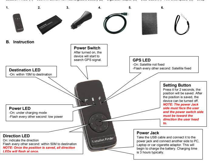
**C.** Look for destination (the position saved before): Turn on the power switch again. The direction LEDs will start to indicate the directions. Following the indication of the direction LEDs, the user can simply find the destination.
